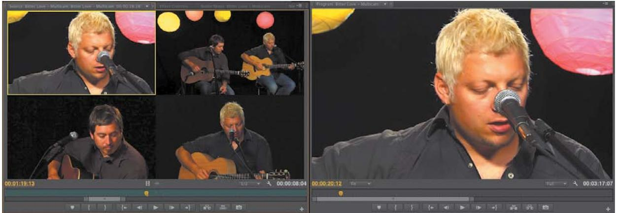
**FIGURE A.11** The yellow border indicates the current angle.
